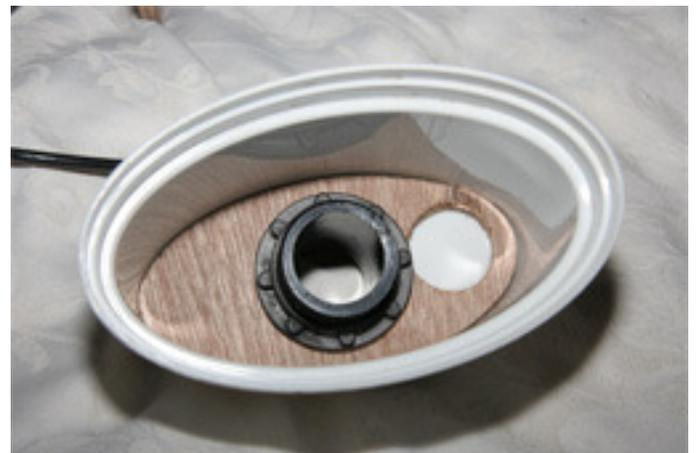
After some gentle sanding and adjustment, I assembled it using Sikaflex as a sealant between the plastic and the wood.
