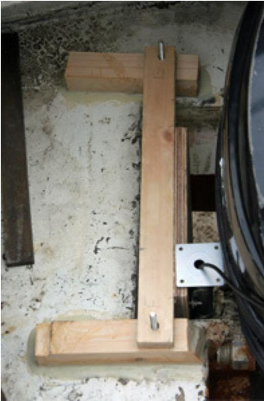
The whole assembly is held tight by 2 M8 wing nuts which are bolted into the bearers.
