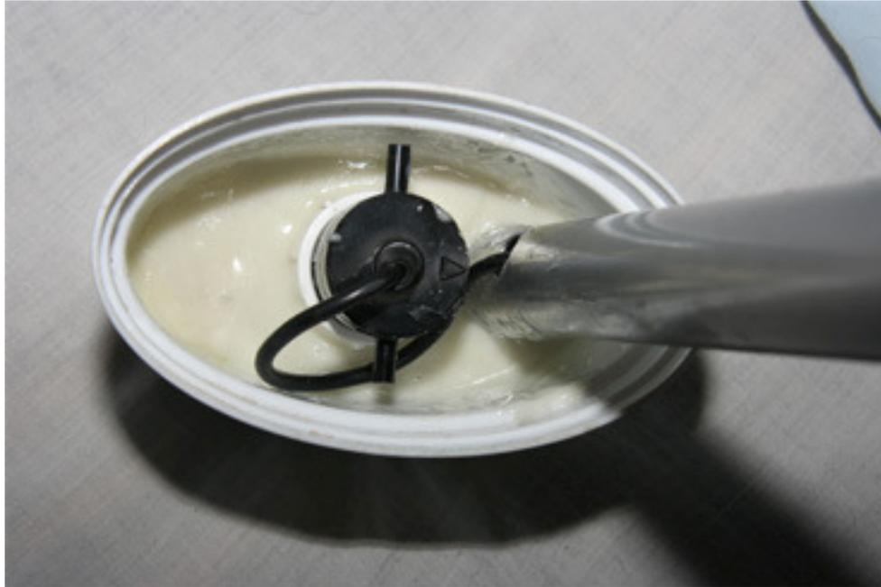
The lid was actually glued into place and sealed with epoxy. A small triangular reinforcement was epoxied to the leg and top.
