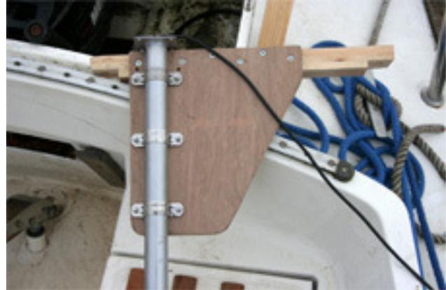
The top of the leg is supported by a crosspiece and a plywood support.
