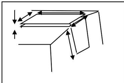
Method: The cover and blind are made separately. Hatches can vary, so I'm going to cop out and tell you to measure your main hatch as shown on the left: Chalk out a rectangle of canvas to slightly greater than the area of the main hatch then add the depth of the hatch and 2" of seam to each side. As
