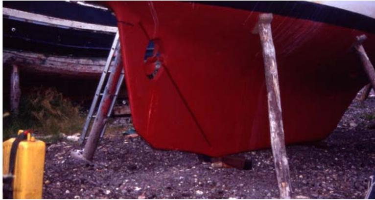
The extension piece was replaced with 38mm square pieces, glued and screwed onto the rudder then each other then faired down by hand. New steel straps were added but they are probably there to reinforce the confidence in the repair more than the rudder, mahogany laminated with epoxy is more than strong enough on its own. Some years later the strips were seen to have rusted, but the repair had not shifted in the slightest. The finished shape is shown above.
