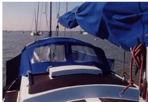
independently attached to the coachroof. In both cases the forward frames are secured by fabric loops to the roof of the sprayhood. The forward fabric edge on Cyano is secured to the coachroof with press-studs (sketch, below, left). On Andani a cord runs through the hem and is tensioned by a shock-cord passing under the grabrail (photo, below, right). The latter method tensions the edge
