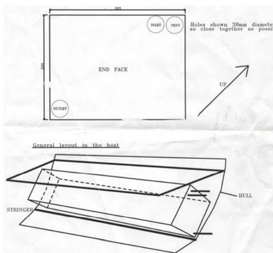
end face. The tank is placed against the hull, so the bottom corner is the position for the outlet, the top corner is the position for the vent and the inlet was placed as high as was possible as shown in the diagram.
